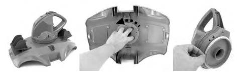
2. Use the screwdriver to unscrew the 4 screws located at the bottom of the head to release the bottom plate first. Then unscrew all the screws at the base as shown. Remove the impeller and pry open the base to expose head inside.
