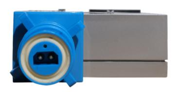
On the output of the swivel if you disconnect the cord going to the cleaner if you turn On the cleaner and if the blue light is On but there is no red light at the output, this means the transformer is OK, the cord between the transformer and the swivel is OK but the swivel is defective (power in is OK but no power out)
