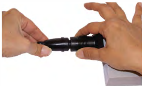
5.4 Slide the cap to contact the plug of the floating swivel union.
