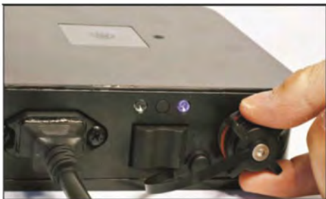
5.1 Unscrew the cap next to the switch.
