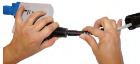
5.3 Insert the end of the floating cable from the transformer into the black "POWER" socket. Be careful with the direction of the plug.
